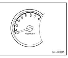
The tachometer shows your engine speed in revolutions per minute (rpm).
